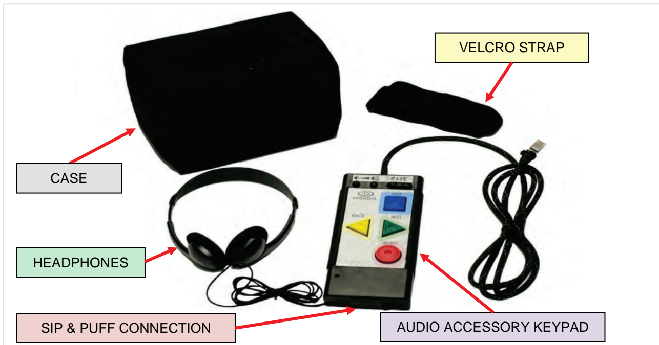
Figure 27: Connect Audio Unit to the Back of the Voting Machine
