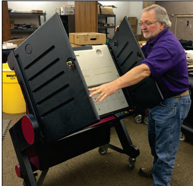
Figure 48: Closing Front Doors of Voting Machine
