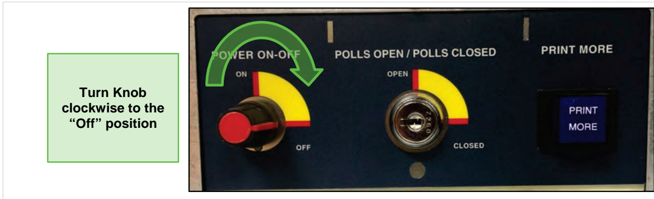
Figure 49: Turn Power Switch to Off
